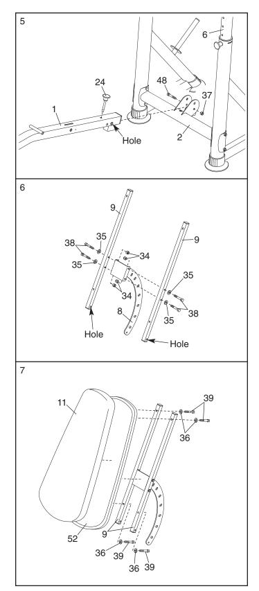
Insert the Adjustment Bracket (8) through the Frame (1) as shown. Apply a small amount of the included grease to an M10 x 168mm Button Bolt (45). Attach the Backrest Frames (9) to the Frame (1) with the Button Bolt, two M10 Washers (49), and an M10 Nylon Locknut (37). Do not overtighten the Nylon Locknut; the Backrest Frames must pivot easily.
